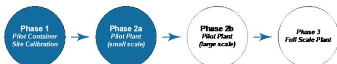
Phase 1 is designed to calibrate the performance of the membrane at Holcim’s plant with the actual flue gas stream following which the up-scaling will then occur in two stages to demonstrate that the performance of the membrane is maintained with increased scale.
